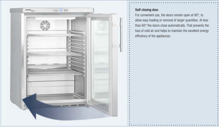
For convenient use, the doors remain open at 90°, to allow easy loading or removal of larger quantities. At less than 60° the doors close automatically. That prevents the loss of cold air and helps to maintain the excellent energy efficiency of the appliances.
