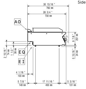
EI = Electrical inlet (power) EQ = Equipotential screw
