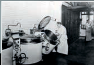
First generation of tilting boiling pans 1934
