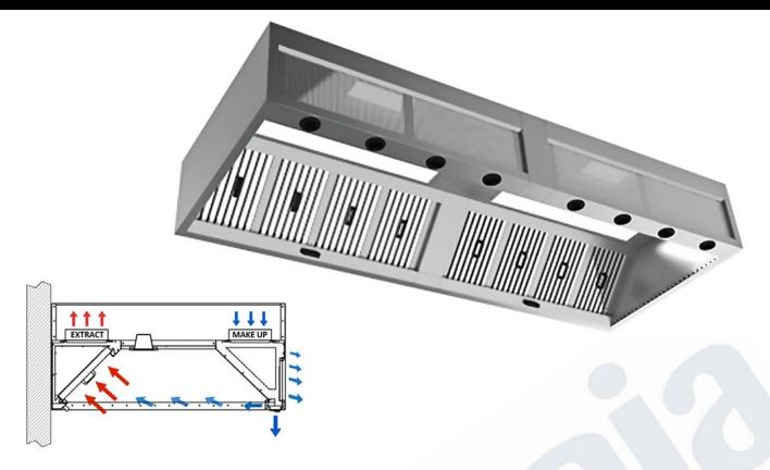
Britannia Capturestream 'CS3' Canopies offer total control over make-up air by providing diffused air to the front, spot cooling and the patented '*Capturestream*' of air across the canopy from the front and two sides for superior performance through intelligent design and world-class baffle filter technology, all contributing to lower exhaust air rates.
