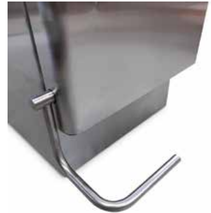
Foot switch for mixing when tilting releases hands.
