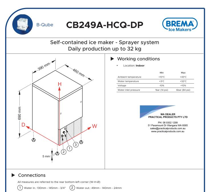
3 Electrical connections.: 95mm - 209mm
