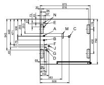
A Water connection (for boiler)
