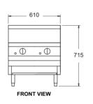
**MODEL: RBA-24L Specifications:** Dimensions (WxDxH): 610 x 800 x 715 mm Working Height: 500 mm Grill Size (WxD): 508 x 546 mm 114 kg 19 mm BSP Weight: Gas Connection: Rating: 76 mj Packed: 0.3 m<sup>3</sup>
