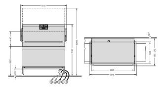
Maximum table profile height with AMXXL and AUPL in corner installation: 40 mm.
