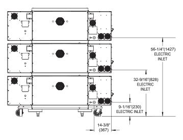
PS640 Back View – Electric Triple Stacked w/Outriggers
