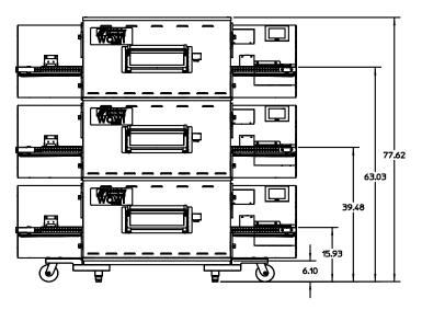
PS640 Front View – Electric & Gas Triple Stacked w/Outriggers
